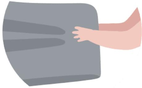
Lay flat and run your fingers along the wire. Pay special attention to the top and bottom of the blanket where the wire bends. If any portion of the wire is twisted on itself, manually twist it back
