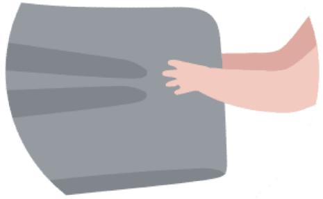
Lay flat and run your fingers along the wire. Pay special attention to the top and bottom of the blanket where the wire bends. If any portion of the wire is twisted on itself, manually twist it back
