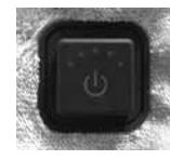
5 Heat setting switch. Continually press switch and the Led's will light as the heat level gets higher.
