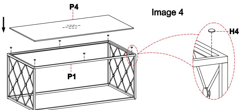
ADDITIONAL NOTE ABOUT SAFETY: BOLTS MAY LOOSEN DURING NORMAL EVERYDAY USE. THEY SHOULD BE PERIODICALLY INSPECTED AND RE-TIGHTENED TO PREVENT DAMAGE OR INJURY. ALWAYS CHECK TO ENSURE THAT ALL HARDWARE IS KEPT TIGHTENED.
