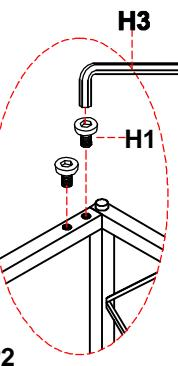
Step 2. Loosely attach the other side frame (P2) to the assembled top frame (P1) and stretcher (P3) as shown on below image 3.
