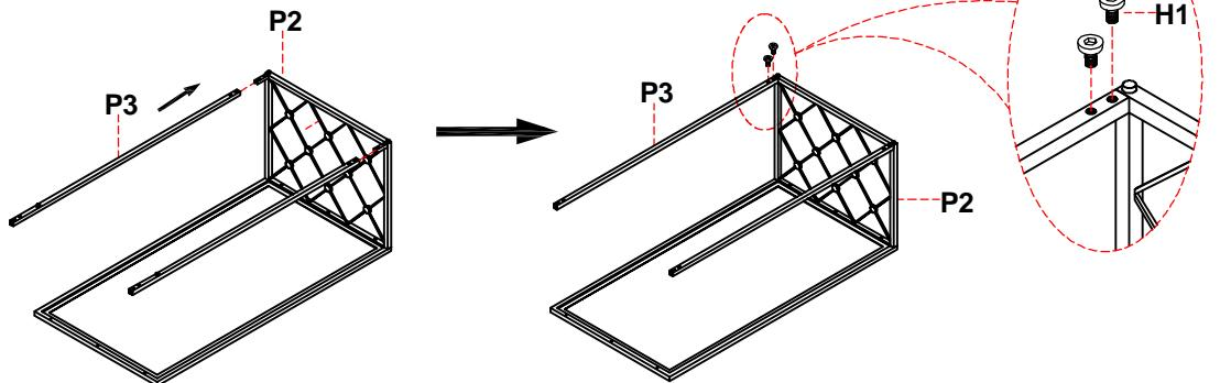
Step 3. Loosely attach the other side frame (P2) to the assembled top frame (P1) and stretcher (P3) as shown on below image 3.
