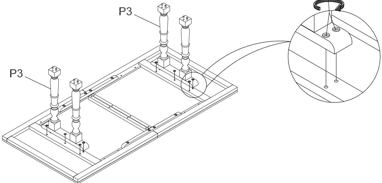
Step 5: Attach the Base Frame assembled in Step 3 to Leg Frames (P3) as shown below then tighten all Bolts.
