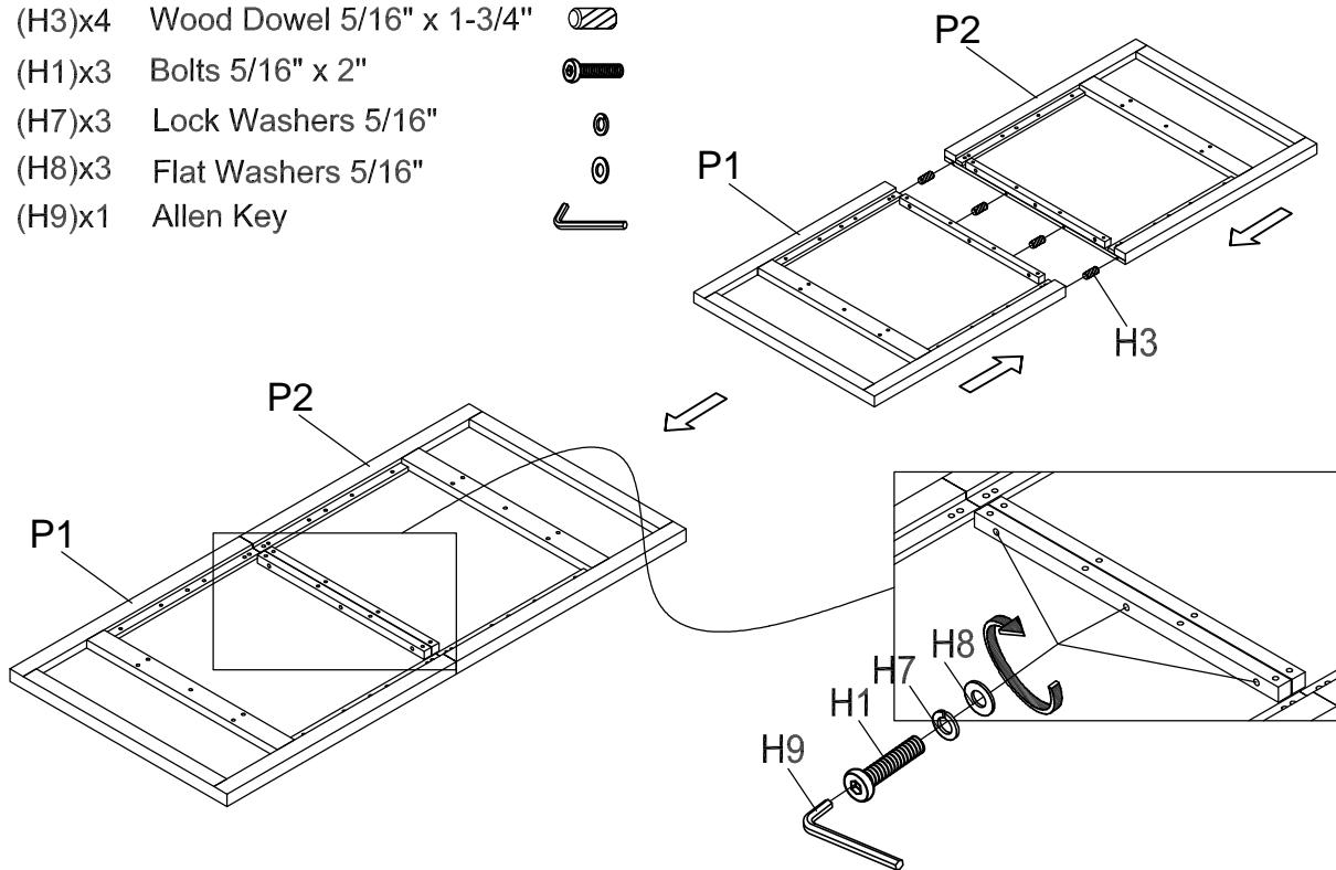
Step 2: Attach the Support Rail (P7) to the Table Top (P1) & (P2) as shown below.
