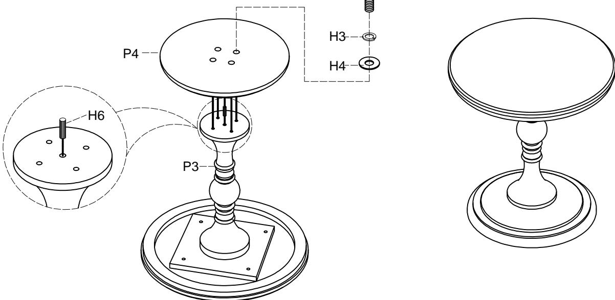
**ADDITIONAL NOTE ABOUT SAFETY: BOLTS MAY LOOSEN DURING NORMAL EVERYDAY USE. THEY SHOULD BE PERIODICALLY INSPECTED AND RE-TIGHTENED TO PREVENT DAMAGE OR INJURY. ALWAYS CHECK TO BE SURE THAT ALL HARDWARE IS KEPT TIGHTENED.**
