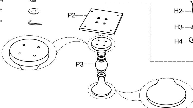
Step 2. Attach the assembled counting plate (P2) to the table top (P1) as shown below image 2.
