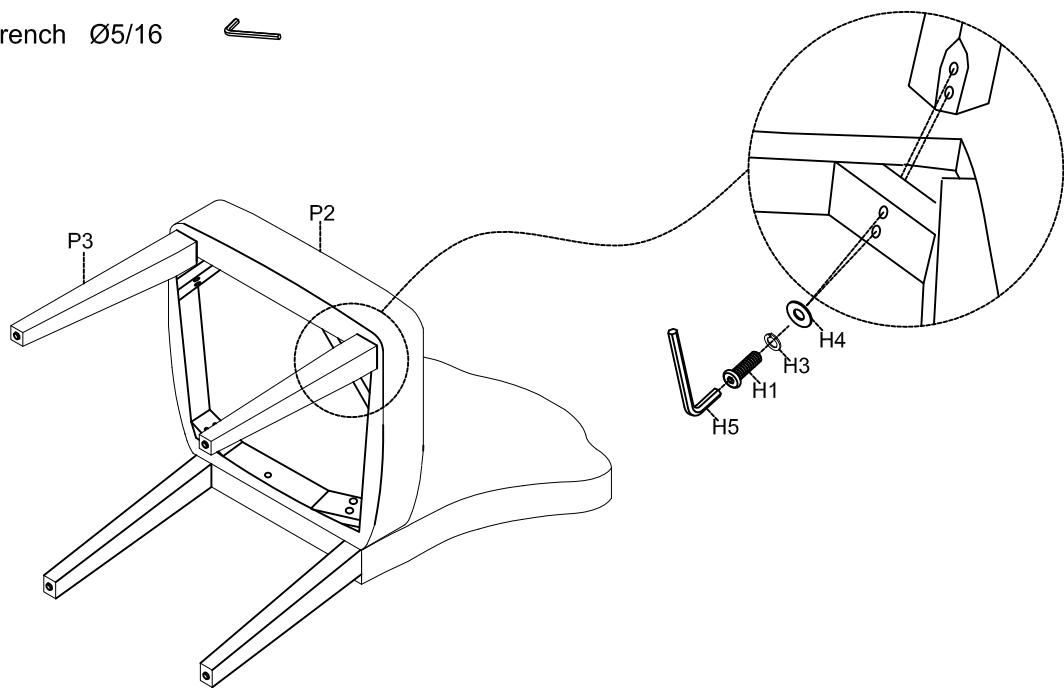
Step 3. Securely tighten all bolts with Allen wrench(H5). Turn the assembled chair to an upright position, make sure the chair is level, aligned properly. Assembly is complete. **Failure to follow these instructions may cause the bolts to misalign during assembly.**
