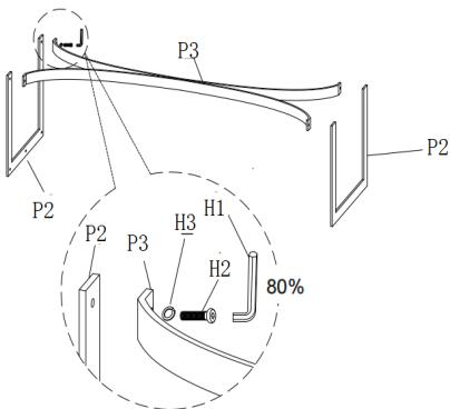
Step 2. Using bolts (H2), Spring washer (H3), attach legs (P2) to bench top (P1). Tighten bolts (H2) with allen wrench (H1) as illustration below.
