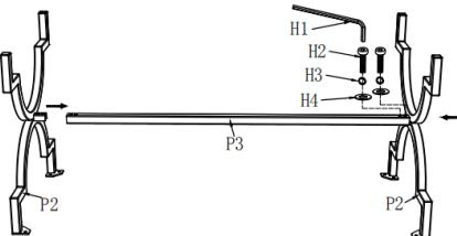
Step 2. Using bolts (H2), lock washers (H3), flat washers (H4), attach legs (P2) to bench top (P1). Tighten bolts (H2) with allen wrench (H1) as illustration below.
