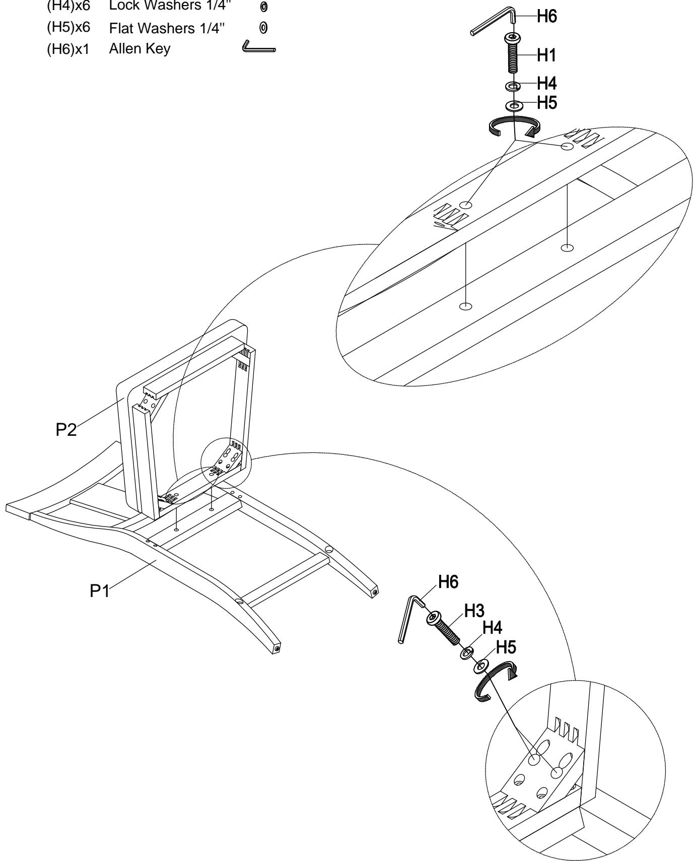
Step 2: Attach the Front Leg (P3 & P4) to the Seat Frame (P2) as shown below and do not tighten bolts.
