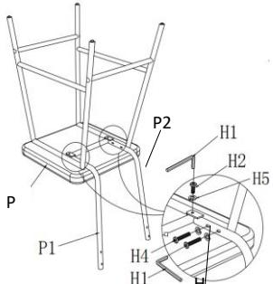
Step 2. Attach the backrest(P4) to the support bar(P1)(P2) with bolts(H3),tighten the bolts securely with Allen wrench(H1) as illustration.
