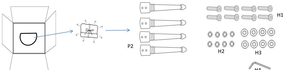
Step 2. Using bolts (H1), lock washers (H2), flat washers (H3), connect legs (P2) to ottoman (P1). Tighten bolts (H1) with allen wrench (H4).
