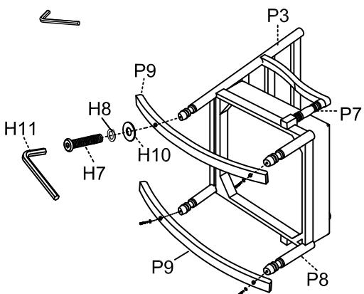
Step 6. Securely tighten all bolts. Turn the assembled chair to the upright position.
