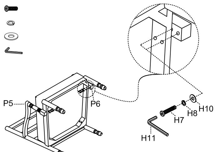
Step 4. Attach the left arm (P5) and right arm (P6) to the back frame (P3) as shown below.
