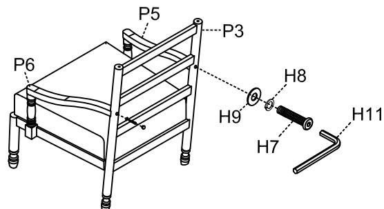
Step 5. Attach the bottom rail (P9) to the assembled back frame (P3) and front legs(P7,P8) as shown below.
