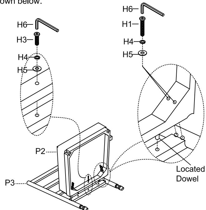
Step 2. Attach the left front leg (P7) and right front leg (P8) to the seat (P2) as shown below.
