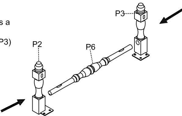
Step 2. Attach the left front leg (P2) and right front leg (P3) to the chair body (P1) as shown below.
