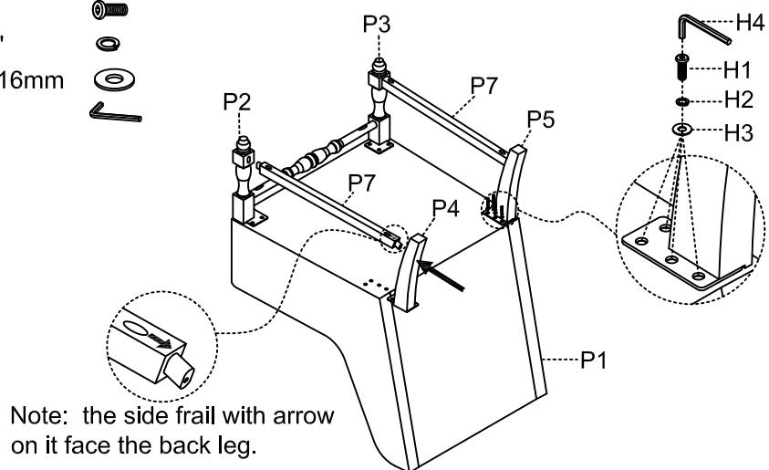
Step 4. Screw the screw (H5) through the front rail (P6) and side rails (P7) to the legs (P2, P3, P4 &P5). Securely tighten all bolts. Turn the assembled chair to an upright position. Assembly is complete. **Failure to follow these instructions may cause the bolts to misalign during assembly.**
