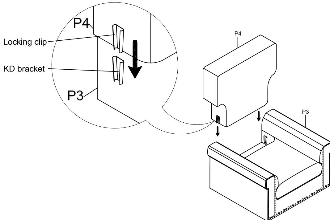
Step 4: Unzip the non-woven fabric under the Chair Top (P4) and assemble the Chair Back to chair top frame using Plastic Head Bolt (H5). Then zip the non-woven fabric.
