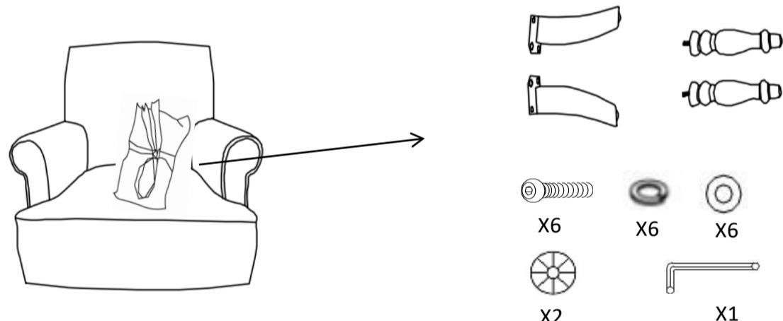
Step 2.Using bolts (H1), lock washers (H2), flat washers (H3), attach back legs (P1&P2) to chair seat (P4).Tighten bolts (H1) with allen wrench (H4). Place washers(H5) on legs(P3) and attach to base by screwing clockwise into corresponding holes.
