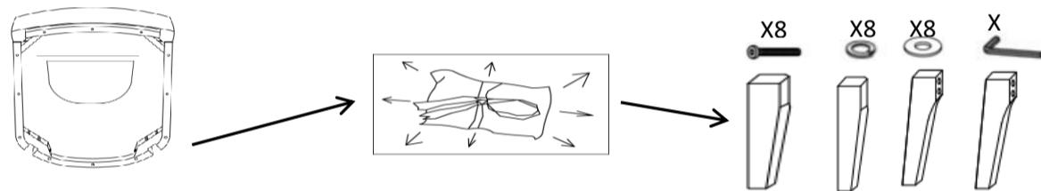
2. Using bolts (H1), lock washers (H2), flat washers (H3), connect legs (P1, P2) to chair (P3). Tighten bolts (H1) with Allen Wrench (H4).
