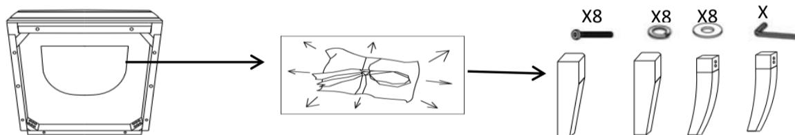
2. Using bolts (H1), lock washers (H2), flat washers (H3), connect legs(P1,P2) to chair (P3). Tighten bolts (H1) with Allen Wrench (H4).
