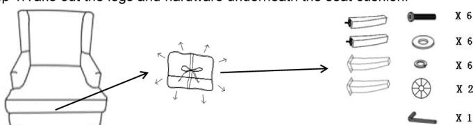
Step 2. Place plastic washer (H1) on front leg (P1) and attach to chair base (P4) by screwing clockwise into corresponding holes. Attach right back leg (P2) and left back leg (P3) with bolt (H4), lock washer (H3), flat washer (H2) to seat frame (P4). Tighten the bolts (H4) with allen wrench (H5).
