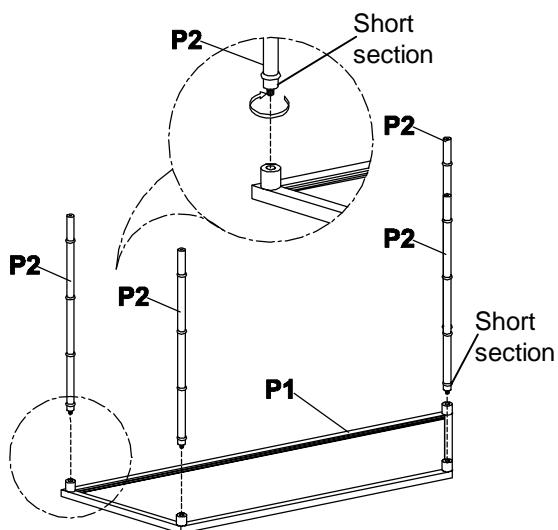
**Step 2.** Attach feet (P4) to the post (P2) through the shelf frame (P3) as shown below. Securely tighten the feet (P4).
