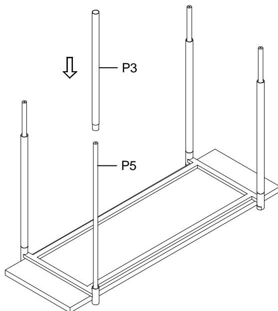
Step 3. Insert the interior post (P5) to the stretcher (P2) as shown below.
