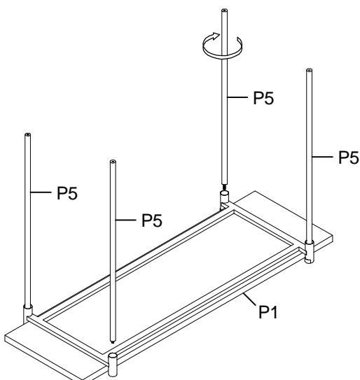
Step 2. Insert the interior post (P5) to the posts (P3) as shown below.
