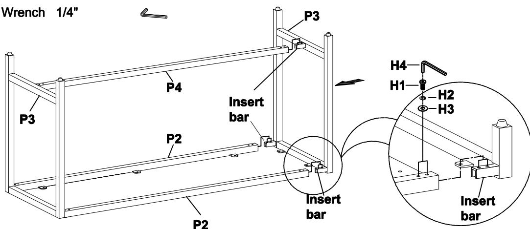
Step 2. Attach the base to the bottom of table top (P1) as shown below. Securely tighten the bolts with Allen wrench (H4) .
