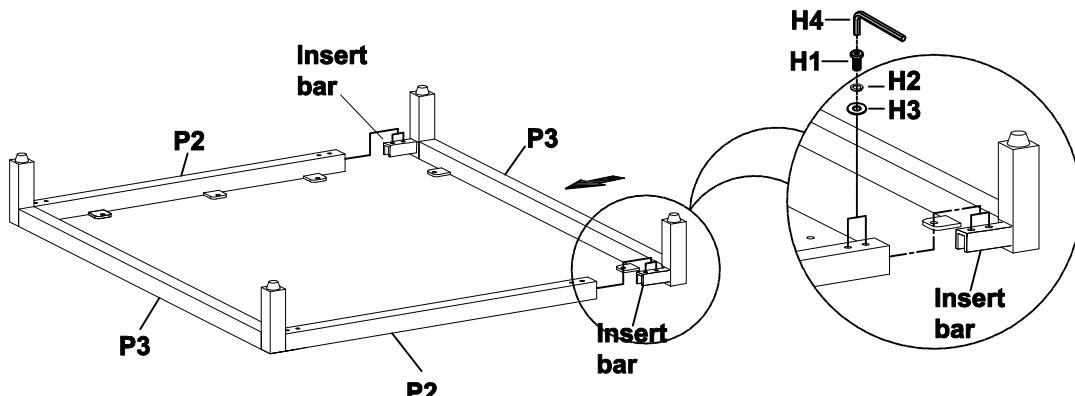
Step 2. Attach the base to the bottom of table top (P1) as shown below. Securely tighten the bolts with Allen wrench (H4) .
