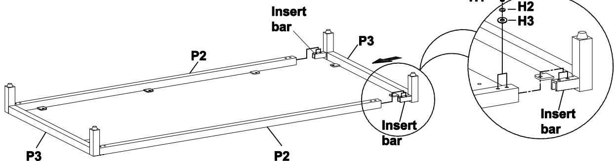
Step 2. Attach the base to the bottom of table top (P1) as shown below. Securely tighten the bolts with Allen wrench (H4) .
