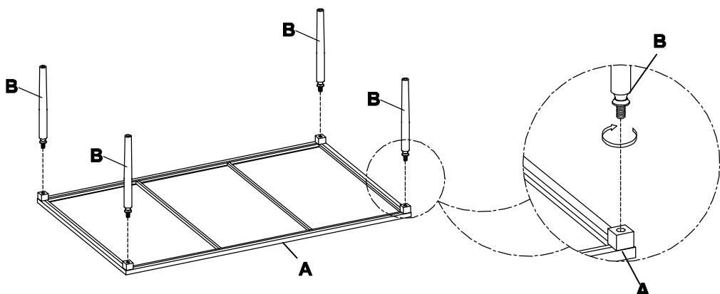
**Step 2.** Attach each foot (D) to the bottom of post (B) through stretcher (C) as shown below. Securely tighten the feet (D).
