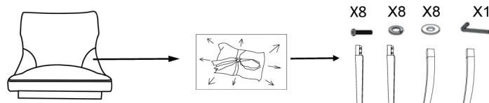
Step 2. Using bolts (H1), lock washers (H2), flat washers (H3), connect legs(P1,P2) to chair (P3). Tighten bolts (H1) with Allen Wrench (H4).
