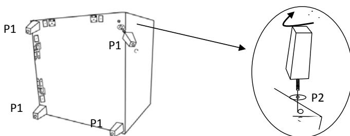
Step 3. With the philips head screwdriver(not attached) remove the screws holding each of the plywood end blocks. Level and put the chair upright on a flat surface, put the Seat Cushion(P4) on the chair.
