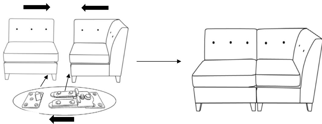
Step 5. Lift the left chair and separate the metal connector. Separate the chairs.
