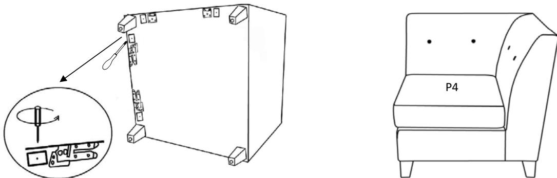
Step 4. Insert the small metal on the bottom into the prefabricated slide lock gadget on the bottom as shown above.
