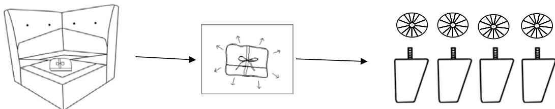
Step 2. Turn the corner over ,screw in the legs (P1) using Plastic Washer (P2) for each. Screw tight to the right angle.
