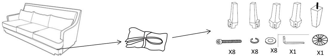
Step 2. Place sofa(P9) upside down onto a protective cloth. Open black fabric on the bottom of sofa. Using bolts (H1), lock washers (H2), and flat washers (H3), connect legs(P1,P2,P3) to sofa . Tighten bolts (H1) with Allen Wrench (H4). Replace black fabric.
