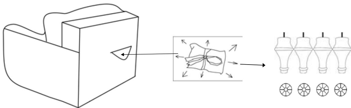
Step 2: Screw in the legs(P2) into the screw hole underneath the base ,using the plastic washers (H1) by rotating legs clockwise.
