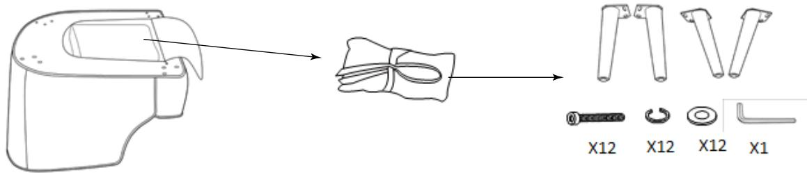
Step 2: Using bolts (H1), lock washers (H2), flat washers (H3), connect legs(P1,P2,P3) to chair (P4). Tighten bolts (H1) with Allen Wrench (H4).
