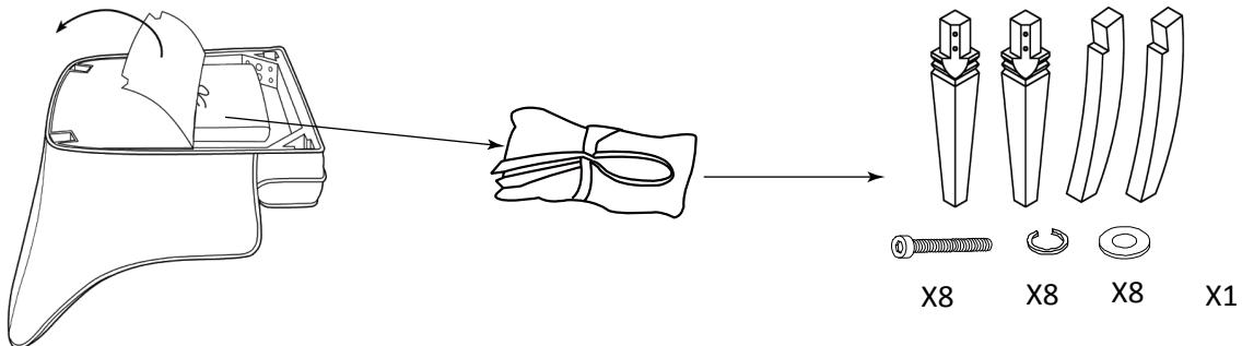
Step 2 :Using bolts (H1), lock washers (H2), flat washers (H3), connect legs(P1,P2) to chair (P3). Tighten bolts (H1) with Allen Wrench (H4).
