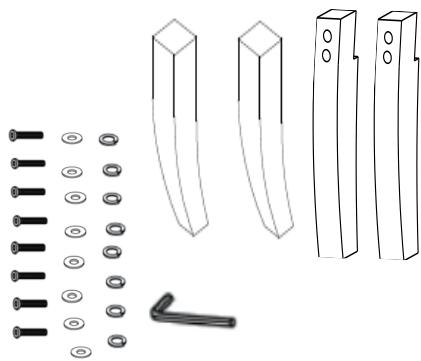
Step 2: Attach the legs (P2,P3) to the seat frame by using flat washer(H3) lock washer (H2) and bolts (H1) ,securely tighten all bolts with allen wrench(H4) ,then sticky the black non-woven fabric .
