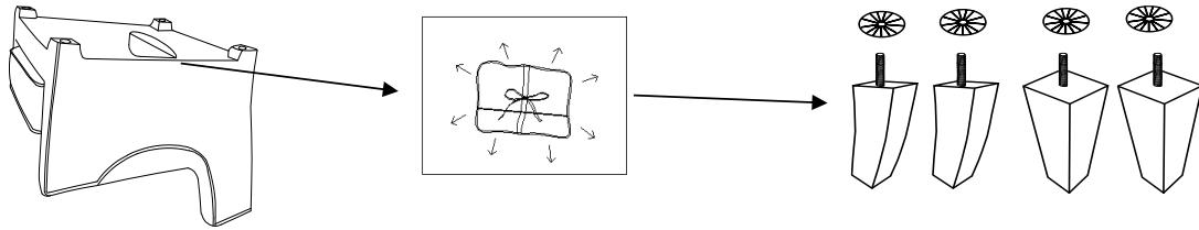
Step 2. Screw in the front legs (P1) and back legs (P2) using Plastic Washer (P3) for each. Screw tight to the right angle.
