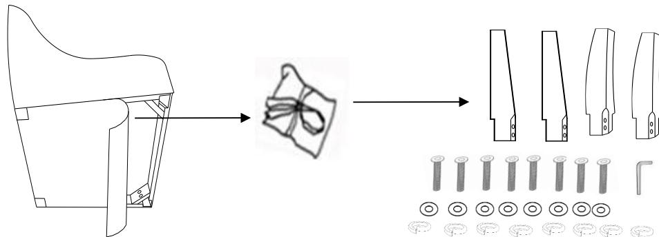
Step 2: Using bolts (H1), lock washers (H2), flat washers (H3), connect legs(P2,P3) to chair (P1). Tighten bolts (H1) with Allen Wrench (H4). Close the black fabric on bottom .
