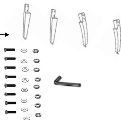
Step 2:Attach the legs (P2,P3) to the seat frame by using flat washer(H3) lock washer (H2) and bolts (H1) ,securely tighten all bolts with allen wrench(H4) ,then sticky the black non-woven fabric .
