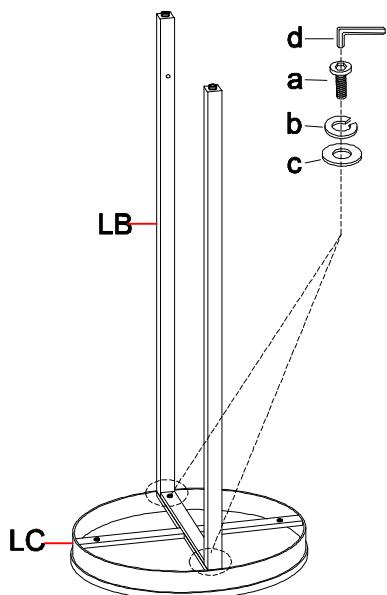
Step 2. Attach leg 1 (LA) to pedestal top (LC) with label " LB" using bolts (a), lock washers (b) and flat washers (c). Loosely tighten all bolts by Allen wrench (d) as shown below.
