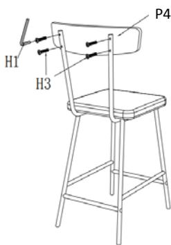
Step 3. Place counter stool upright on a level surface. Adjust levelers (as drawing) as necessary.
