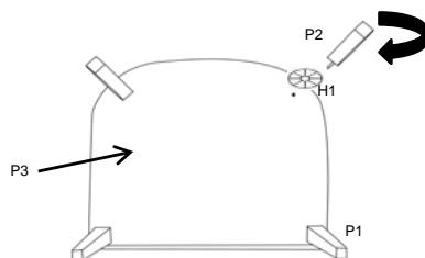
Step 3. Place the chair upright on a level surface. Put seat cushion (P4) on the chair. Assembly is complete.
