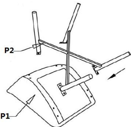
**Step2.** Screw legs with bolt H1 and washer H2,securely tighten all bolts with Allen Wrench H3.
