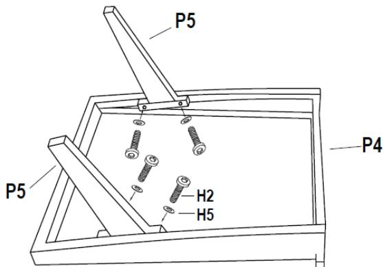
Step 2 .Turn back seat (P2) to the bottom, and lock the P1 on P2 with H2 and H5 .
