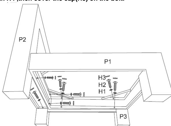
**Step2.** Place the backrest(P3) against the (P1) and (P2) ,fix backrest(P3) to Backrest1(P2) by using H1, H2 ,screw tight with H4 ,then cover the cap(H3) on the bolt.
