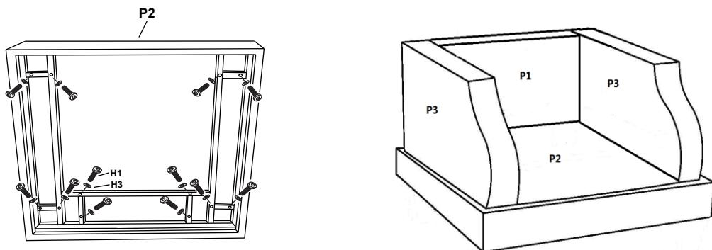
Step3. Lock the legs(P4) at the seat bottom by using Bolts (H2) and washer(H3) .
