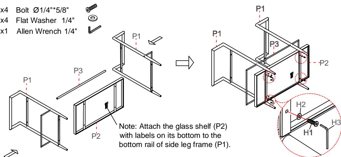
Step 2. Attach the glass shelf (P2) to the assembled side leg frame ( P1) as shown below. Tighten all bolts with Allen wrench (H3) .
