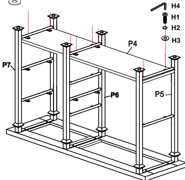
Step 3. Attach medium shelf (P3) and small shelves (P2) to each frame (P5,P6,P7) using bolts (H1), lock washer (H2) and flat washers (H3) as shown below.
