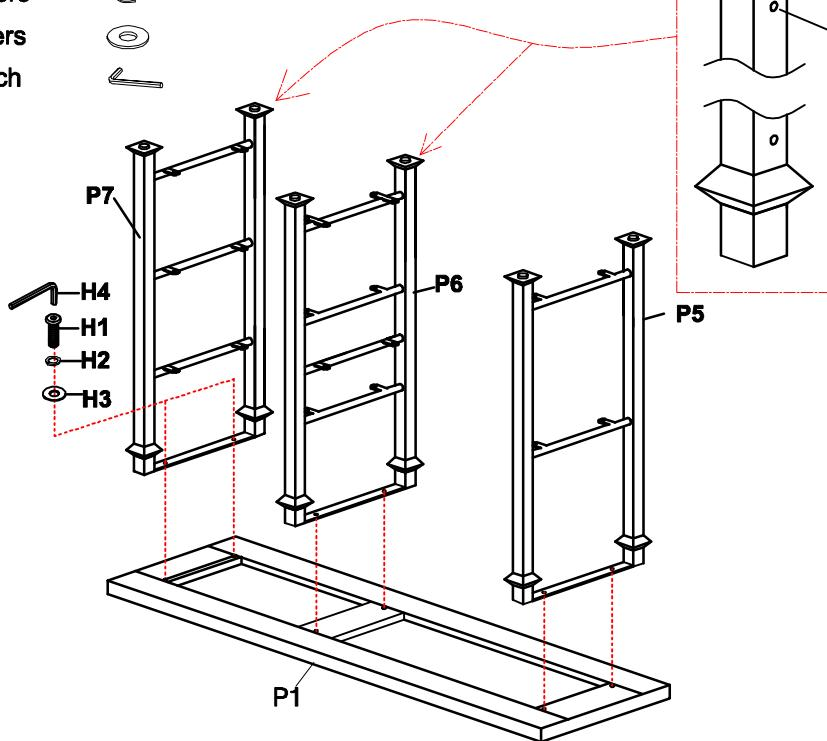
Make sure the holes on right leg frame (P7) and the middle leg frame (P6) on same side.
