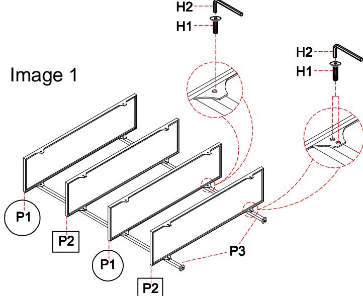
Step 2. Attach the other two support posts (P3) to the assembled shelves (P1&P2) as shown below image 2. Securely tighten all bolts with Allen wrench (H2) .
