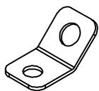
1. Locate a wall stud behind your furniture. Position a bracket on the stud approximately 1" below the top frame of the furniture. Mark and drill pilot hole into the center of the stud with a 3/32" drill bit. Attach a bracket to the stud with the long screws provided.
