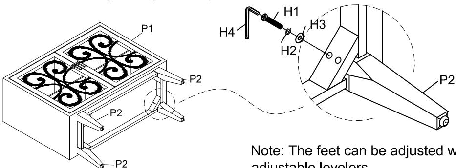
Note: The feet can be adjusted with adjustable levelers.
