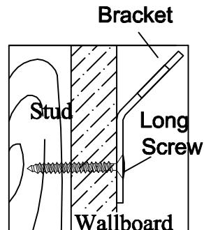
3. Move the furniture into its final position, taking care to line up the wall bracket with the furniture bracket. Thread a strap through the bracket as shown in the illustration. Tighten strap until snug. Do not overtighten.
