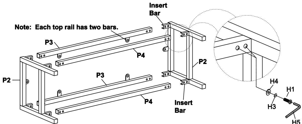
Step 2. **Loosely** attach the assembled base to the bottom of the chest (P1) using bolts (H2), lock washers (H3) and flat washers (H4) as shown below
