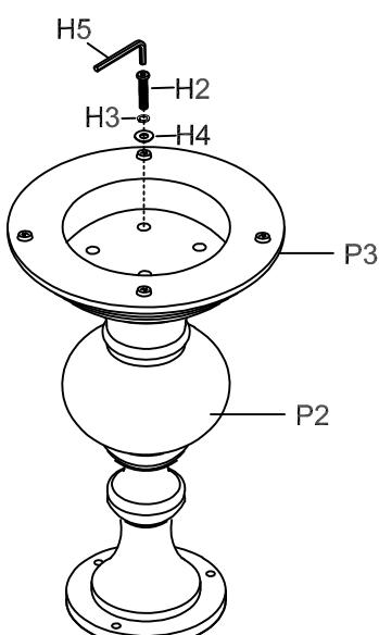
Step 2. Loosely attach assembled post (P2) and base (P3) to the bottom of top panel using bolts (H1), lock washers (H3) and flat washers (H4) as shown below.
